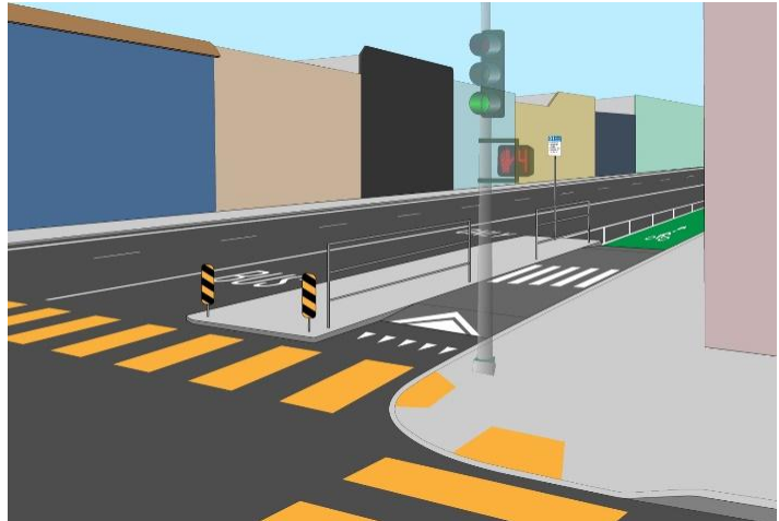
Bus boarding island example diagram with a platform separated from the sidewalk by a bike lane (source: CSET).
