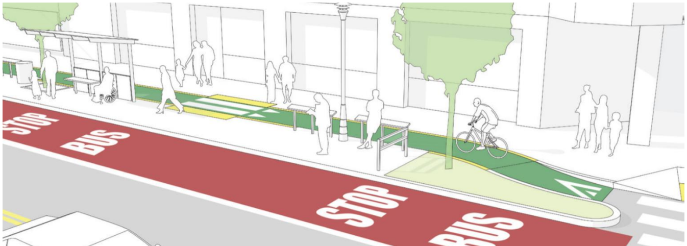
Bus boarding island rendering for San Pablo Avenue in Alameda County (source: ACTC).
